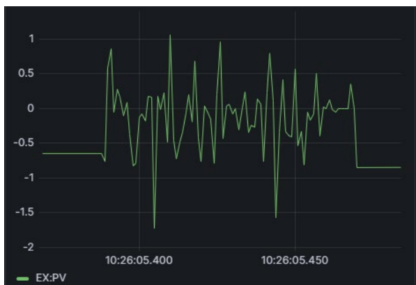
Figure 6: Visualized array data with dt-space format in short time range. This plot roughly shows waveform of the array data. However, it cannot show the index number of each element.
