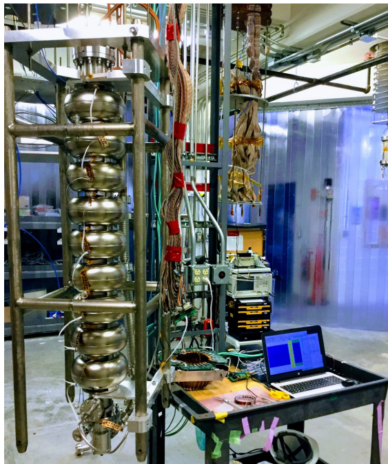
Figure 3: Offline test of sX-map before the vertical test of a superconducting cavity at JLab.
