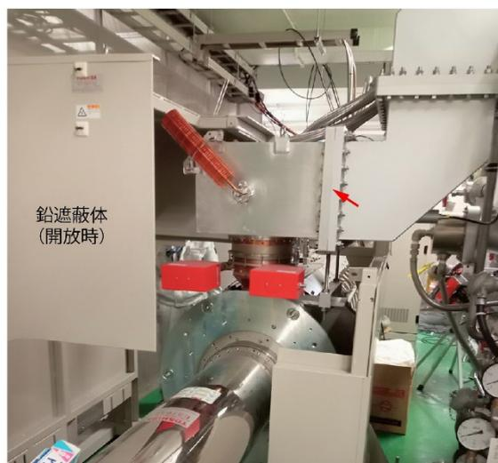
Figure 7: A photograph of a leakage point of the RF at the connection of the rectangle waveguide at the output of the klystron. The leakage point is indicated by a red arrow.
