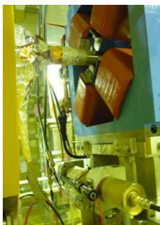
Figure 9: Layout of beam loss monitor.
