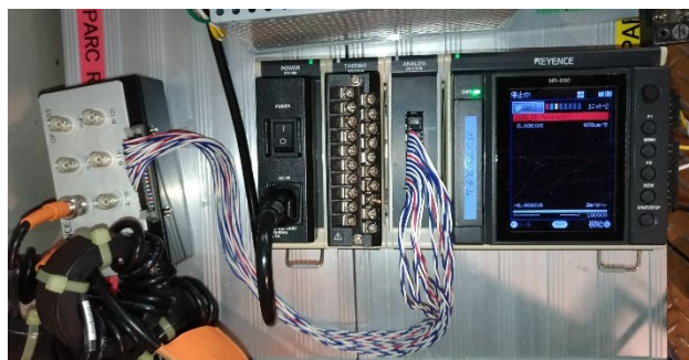
Figure 9: Output voltage monitoring module.
