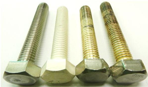
Figure 2: From the left: normal bolt, new, used several times, and used several times and left in the air for a long time Teflon-coated silver-plated bolt (SUS316L).
