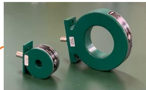
電流測定器 (Pearson Electronics, Model 411 and 110, Bandwidth: 1 Hz - 20 MHz)
