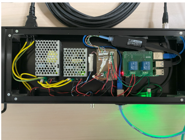
Figure 5: Image of GigE camera controller.
