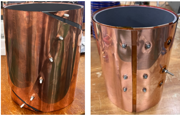
(a) Primary coil (Left: Spiral type, Right: Layer type)
