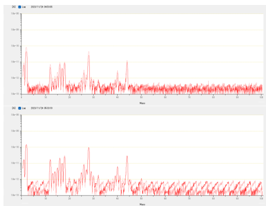
Figure 10: QMS during 260 kW continuous beam operation. (upper) At the beginning of operation, (lower) just before the PC died.
