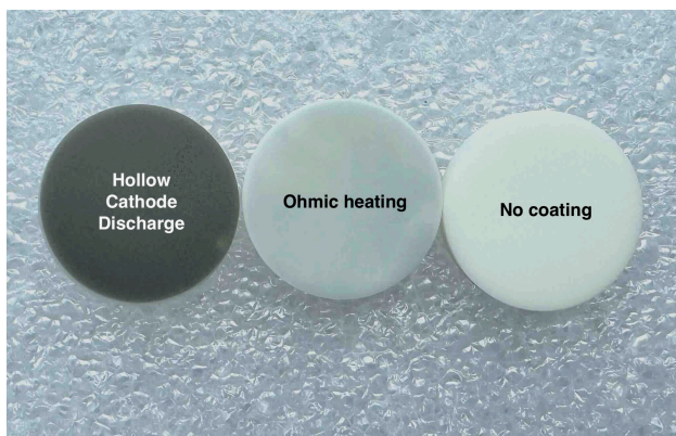
Figure 1: Alumina samples with TiN by hollow cathode discharge, with TiN by ohmic heating, and without TiN coating.
