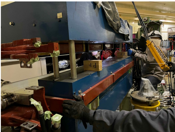
Figure 10: B01 magnet divided in two parts (actually, this photo was taken when the two parts were being put back together.).
