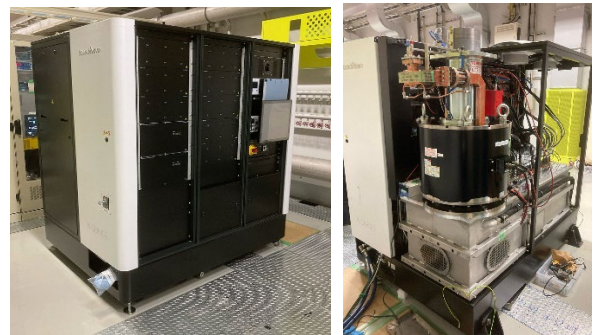
Figure 1: Photograph of the ScandiNova modulator. The C-band klystron is attached to the socket.
