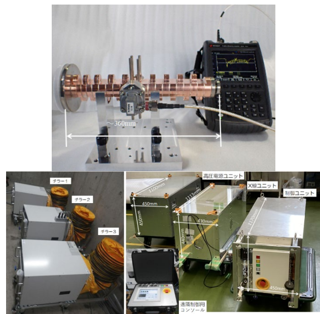
Figure 6: The picture of X-band LINAC and 3.95 MeV small X-ray system. The system consists of three units (X-ray unit, Marx unit, and Control unit) and three small chillers. The operator can control the system remotely using a touch panel PC built into a portable case.
