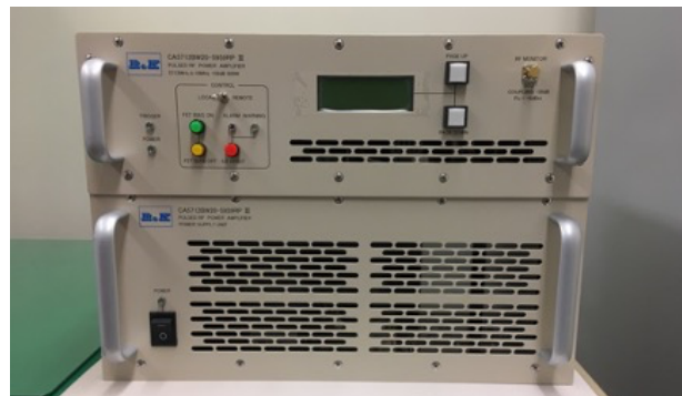
Figure 3: Photo of the 800W solid-state amplifier for a C-band klystron. The top is an amplifier unit, and the bottom is a low-noise power supply unit.
