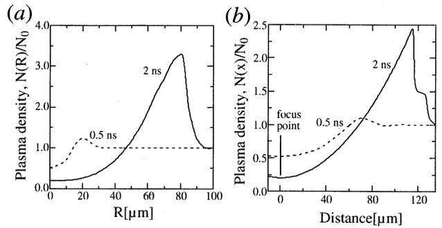
Fig.2 Density distributions of He-jet after the laser prepulse calculated by 2D hydrodynamic simulation. The power density of the prepulse is  $10^{13} \text{Wcm}^{-2}$ , and Rayleigh length is  $50 \mu\text{m}$ . (a) Radial direction ( $z=0$ ), (b) Longitudinal direction ( $r=0$ ).[7]
