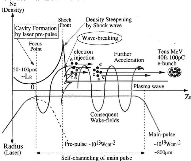
Fig.1 Illustration of electron injection by the wave-breaking at the cavity produced by laser prepulse. The laser pulse is focused by short Rayleigh length optics ( $L_R \sim 50\text{-}100\text{mm}$ ).
