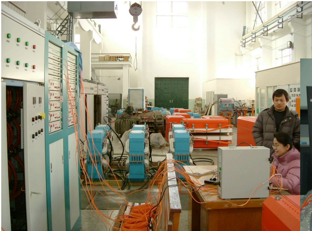
On line test of prototype for chopper PS
